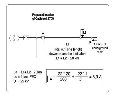
Figure 3. Capacitive discharge current calculation example
