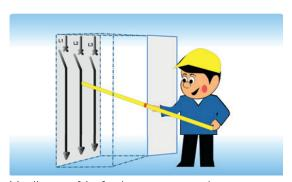
Until now: No fault-arc protection during voltage detection due to open door
