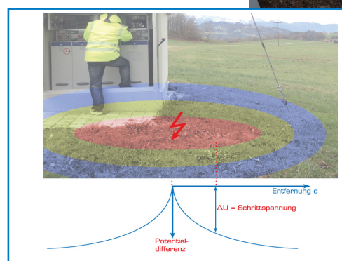
Indication of insufficient grounding or dangerous step voltage in the display. An external LED blinker unit can also be connected to the IKI-23, which is mounted on the outside of the kiosk-station, for example, and indicates the danger.
