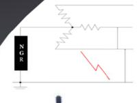
The Neutral Earthing or Grounding Resistors are generally used in the LV and MV distribution networks to protect power transformers and generators from damaging currents in the event of earth fault.
