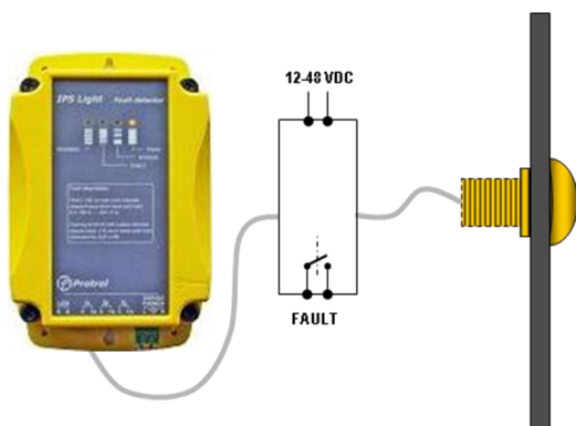
Fig. 8 Relay unit connected to the LED unit cable when both electrical and optical signaling is required
