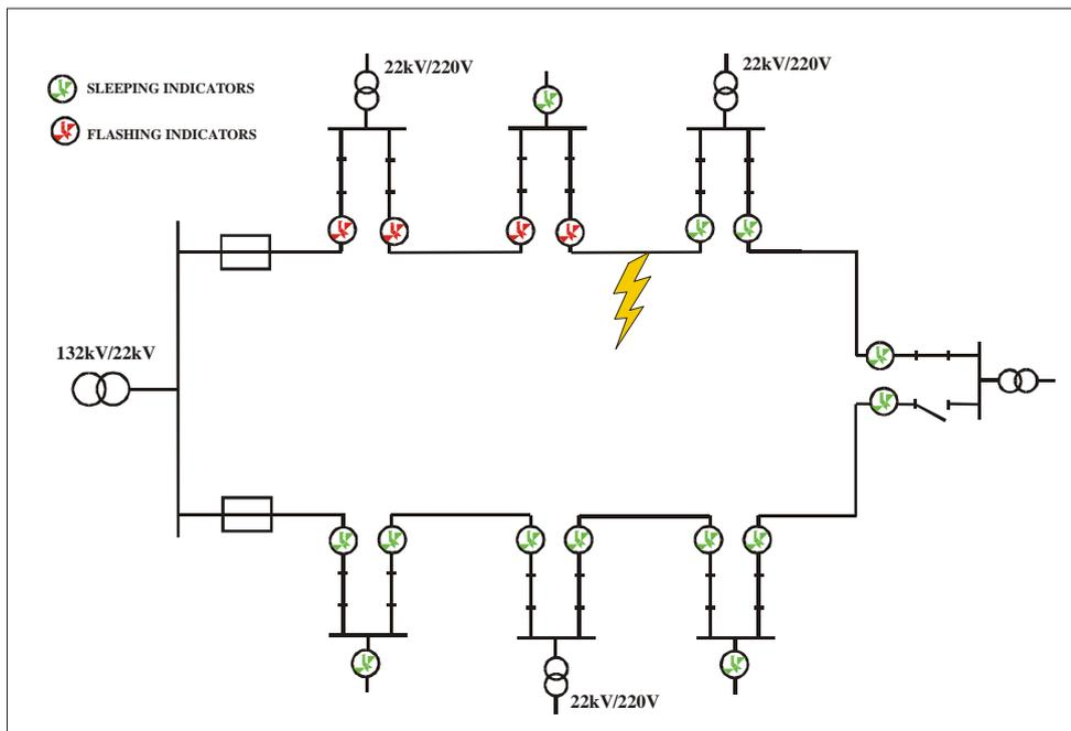
Figure 1. Fault indicator status following a fault
