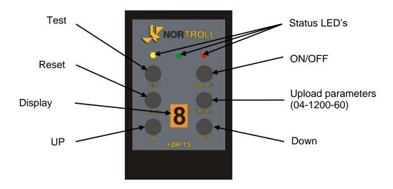
The FDP-15 can be used as a radio interface to a collector or fault indicator when sending configuration data to the unit.
