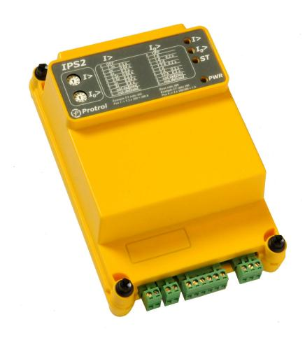
IPS2 is a fault detector for overcurrent and directional earth faults that indicates using its relay output. Supplied by internal supercapacitors, it provides local indication using an external LED for 24 hours without external power supply.
